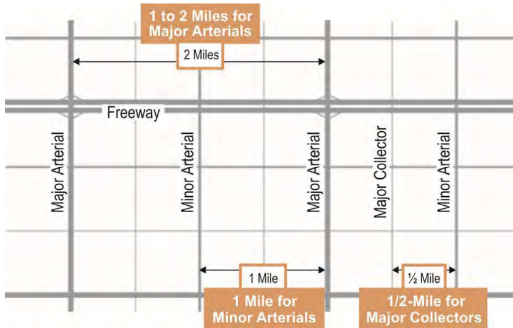
Figure 4: Wilsonville Roadway Spacing Guidelines
