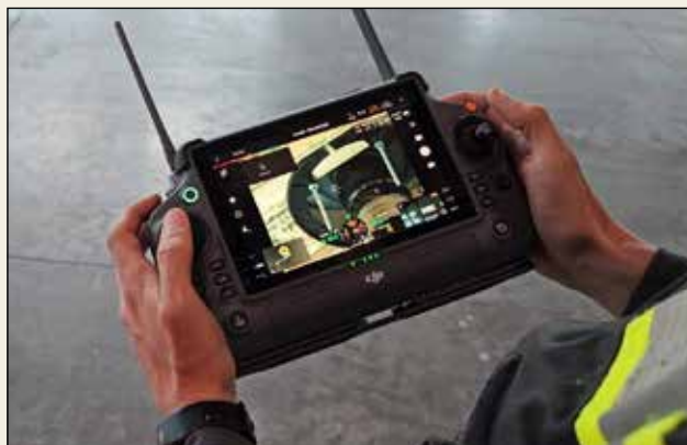
A high-definition control screen gives inspectors an up-close look at hard-to-reach areas.
